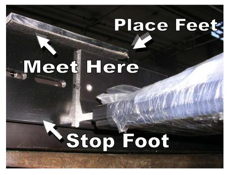
Step (12) Now adjust the stop foot to meet the stop feet.
